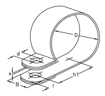
$\begin{array}{ll} d & = 6.4 \\ \text{Diameter D} = 24 \\ \text{h1} & = 21.7 \\ \text{I} & = 6.0 \\ \text{s} & = 0.8 \\ \text{Width B} & = 15 \\ \end{array}$
